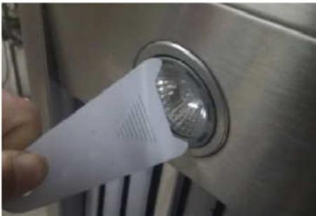
1. Apply the applicator onto the LED unit and turn counter clockwise to release the LED light.
