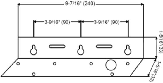
Baffle Filters & Stainless Steel Spacer
